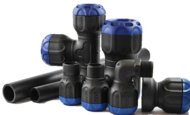
Isiflo Sprint push fittings for extruded PE-pipes according to EN-12201 SDR11 and SDR17 gives a tight and end-load resistant connection. The couplings are easy to use and gives a reliable long-term connection. Assembly without need for special tools.
