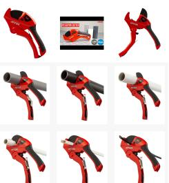
The extremely low friction ration of the PTFE (polytetrafluorethylene) Teflon coating facilitates blade sliding. Cutting load reduced by 20%\*. (\*- 20% on average on different types of tubes compared to a regular coating). Material cut: PVC, PP, PE, PER, PEX, ABS, PEHD, CPVC, PPR, PB, multilayer. Cutting accuracy: the V-shaped blade enables easy, perpendicular cutting. Practical: quick, tool-free blade change.
