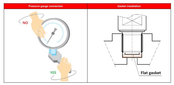
Pressure gauges are maintenance-free, but should be checked at regular intervals to ensure accuracy. Checks and recalibrations should only be carried out by qualified personnel using the appropriate equipment. When dismanting, close the upstream valve.
