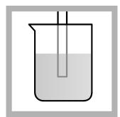
probe in a beaker that contains the solution. Do not let the probe touch the stir bar, bottom or sides of the container. Remove the air bubbles from under the probe tip. Stir the sample at a slow to moderate rate.
