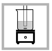
**4.** Put the probe in the solution. Do not let the probe touch the stir bar, bottom or sides of the container. Remove the air bubbles from under the probe tip.
