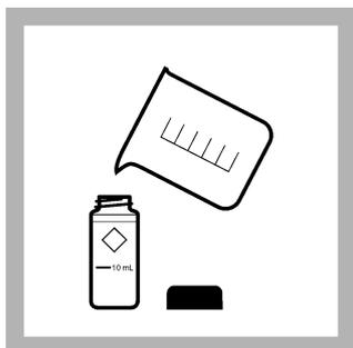
**2. Prepare the blank:** Rinse a sample cell and cap three times with sample. Fill the sample cell to the 10-mL mark with sample. Close the sample cell.
