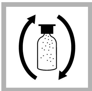
9. Quickly invert the AccuVac Ampul several times to mix.
