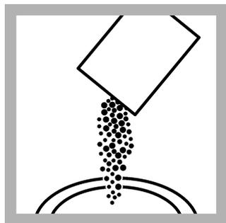
**9. Add one 10-mL DPD Free Chlorine Reagent Powder Pillow or one 10-mL DPD Total Chlorine Reagent Powder Pillow to the second sample cell.**
