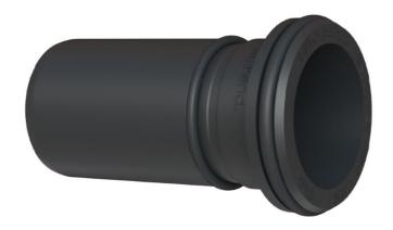
Isiflo Seal Liner is used on SDR11 and SDR17 PE-pipes according to EN-12201 to straighten out ovality, add structural support and extra sealing in the interface between pipe end and Isiflo fitting. EPDM O-rings. The pressure loss using this liner is minimal.
